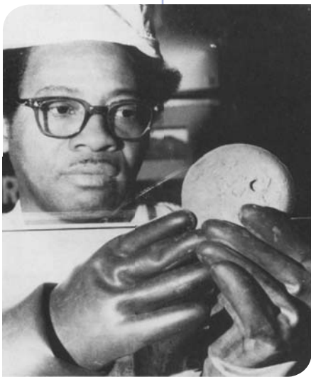
Worker at the Rocky Flats Plant examining a plutonium button inside a glove box designed to protect workers from radiation. Photo: Department of Energy
